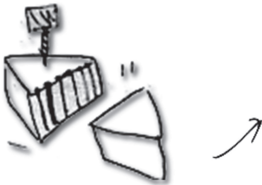
Figure 7. Split Aji stone using feathers and wedges.
