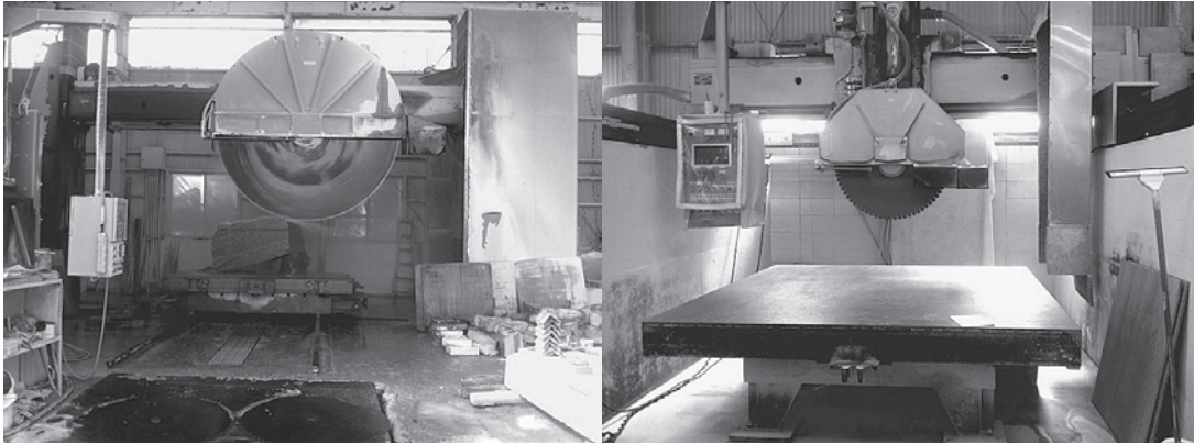
Figure 9. Machines used in the factory to cut Aji stone.
